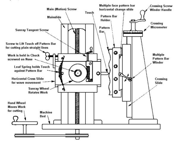
This diagram is intended to show how the workpiece can move vertically on the machine, thus driving a horizontal oscillation generated from the pattern bar
