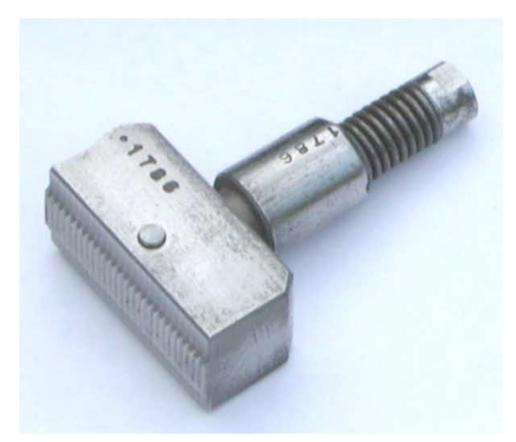
The Pledge Multiple Touch with much stronger spring and hardened ball joint. This example is a 90 degree zig zag that, having been made on an engine turning machine using the same sliderest that is used for engine turning the end product, will produce an exact 90 degree square basket weave for watch dials. It is believed that all examples of this have been sold when the company was liquidated and their wherabouts are unknown
