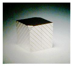
Matching the diagonals on all sides required care both in manufacture and engine turning. Although simple to understand as a design, great skill was required to match the lines to look continuous, whichever way the pair of objects were placed side by side.
