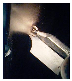
As the workpiece is moved downwards, the stationary tool, with depth of cut limited by the guide, cuts a straight line, removing a curling chip of metal in a straight line.
