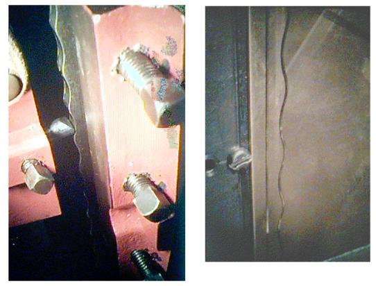
By guiding the vertical path of the workpiece away from a straight line to a wave with a wavy pattern bar we can
