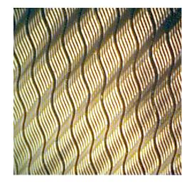
If we move the pattern bar vertically with relation to the workpiece and the machine, in this case 6 times a small amount, then a gap and repeat, we get a diagonal progression
