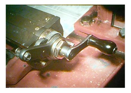
Using the ratchet on the sliderest we can move the tool a little to the right at a time to achieve a series of parallel cuts ...
