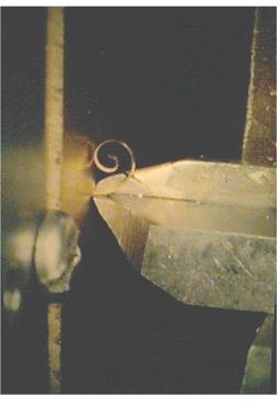
The tool and guide viewed from the left side of the machine. The tool is in the foreground, the guide immediately behind it in this image. The Guide controls the depth of cut by following the surface very close to the edge of the cut. For normal engine turning, The tool and guide are locked together while cutting takes place, though for deep cuts the guide may be withdrawn a fraction at a time as multiple passes of are made in the same cut to achieve the required depth
