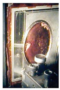
Firstly one must sink around all the holes Then all the edges, and then plane across the main area to lower the surface by about 0 35mm. This is then carefully scraped, stoned and pre polished to provide a clean surface for the engine turning
