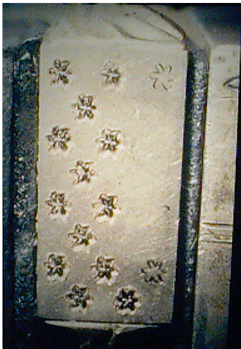
A small pill box for sweeteners in the shape of a wrapped sweet is being recessed with tiny flower shapes about 3mm across for enamel.
